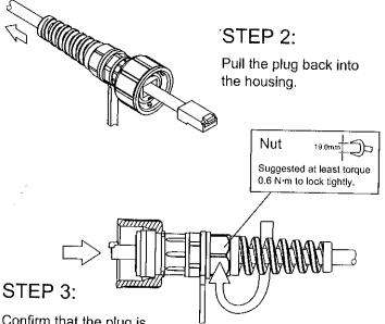
Confirm that the plug is in the correct position.
