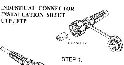
Insert the wire through the parts as shown.
